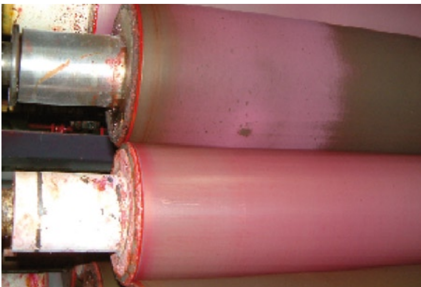
Fig. 3 [top] and Fig 4 [bottom]: The printed sheet [top] clearly shows the impact of the defective rollers in the inking unit.
