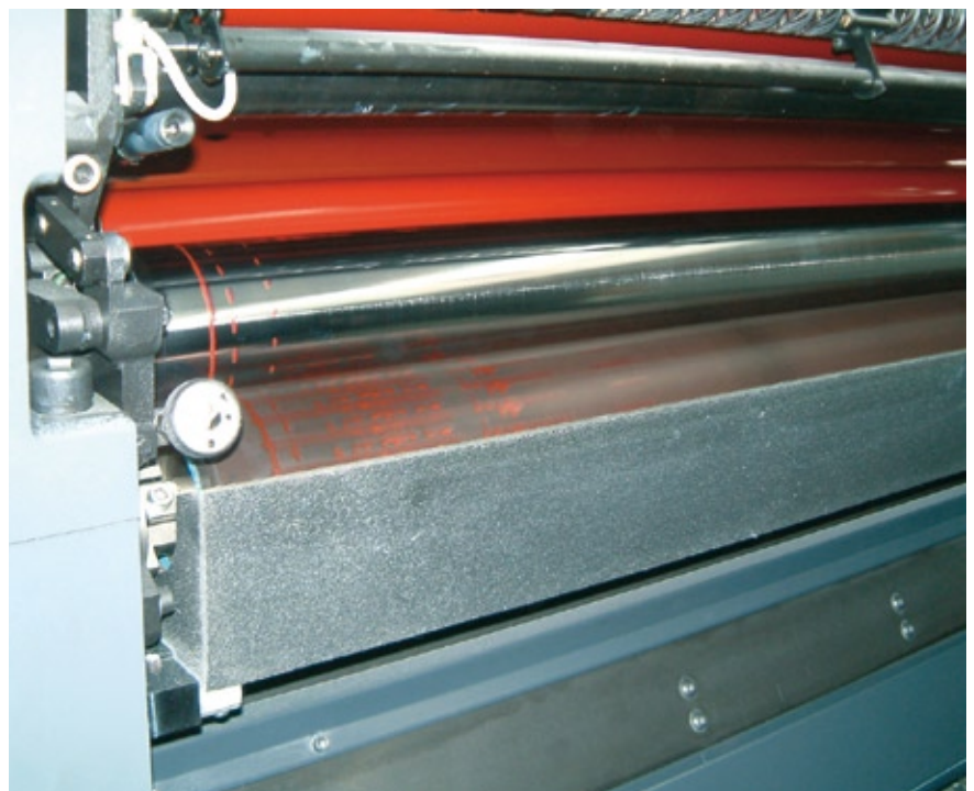
Fig. 6: Ink on chrome rollers in fountain unit after only 100 rotations.
