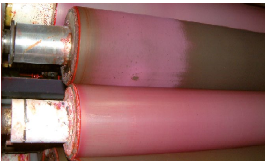
Fig. 3 (top) and Fig 4 (bottom): The printed sheet (top) clearly shows the impact of the defective rollers in the inking unit.
